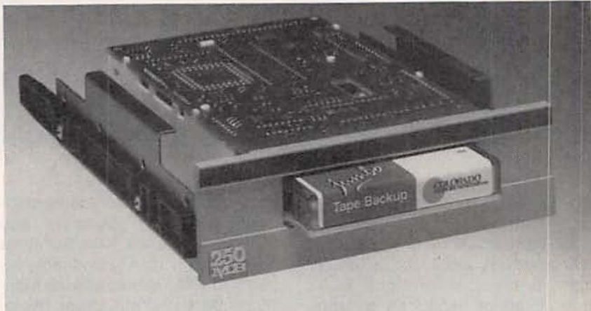
FIG. 1—COLORADO'S JUMBO 250 packs 250 megabytes of data on a $20 tape cartridge in less than two hours.
