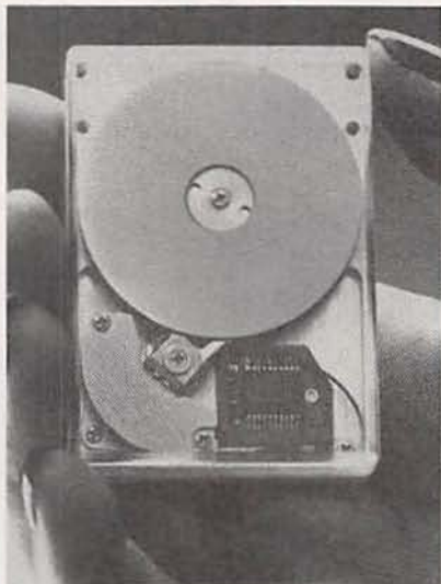
HEWLETT-PACKARD'S 1.3-INCH DRIVE shown here actual size.
