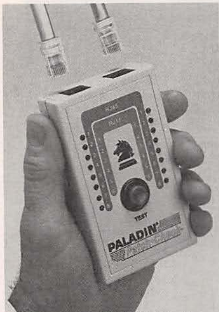
FIG. 3—PALADIN'S PATCH CHECK provides instant go/no-go testing of RJ-11 and RJ-45 telephone-style connectors, used for shielded and unshielded twisted-pair wiring.
